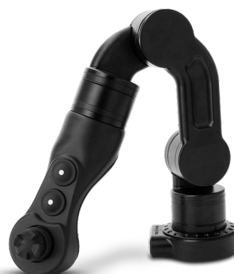
Master Arm for 5-function Reach manipulators RM-5201
