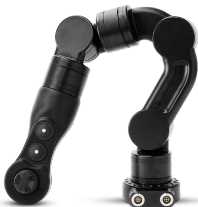
Master Arm for 7-function Reach manipulators RM-7201
