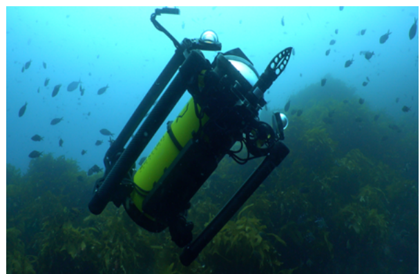
Reach Alpha Grabber integrated on Boxfish ROV during sea trials
