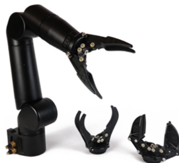
Reach Bravo 5 with Interchangeable End Effector tools
